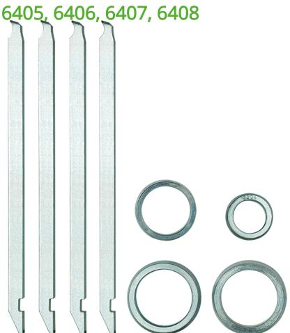
The pulling jaw sets of series 70-S are suitable for bearing pullers of series 70 and are used for non-destructive pulling of ball bearings without removing the shaft. In addition to the pulling jaws, the sets also include support rings as spare parts.
