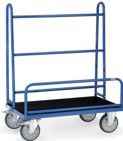
Tubular steel and profile steel welded, powder coated blue RAL 5007. Platform made of derived timber material board, surface covered with corrugated rubber. Bolted tubular steel superstructure. 2 swivel and 2 fixed-wheel castors, TPE tyres, hubs with groove ball bearing. Swivel castors with wheel locks, according to the European Standard EN 1757-3 (safety of platform trolleys). Effective height: 1050 mm, Height retaining bracket: 300 mm.
