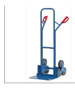
Tubular steel, with lifting blades made of steel plate, sturdy welded construction, powder coated, blue RAL 5007. Safety handles. With 2 three-armed wheel spiders, each equipped with 3 TPE tyres 160 mm Ø. Curved top bar and transversal struts. For safe transport of circular items such as rolls, cans, buckets etc. Steel sheet front shovel mountable. Flat packed delivery.
