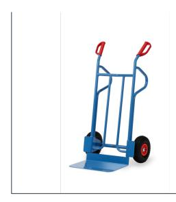
Handy tubular steel trucks with steel sheet blades, sturdy welded construction, blue RAL 5007. Safety grips. Steel sheet front shovel mountable, therefore exchangeable. Pneumatic tyres on synthetic rims, hubs with roller bearings. Flat packed delivery.
