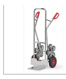
Aluminium tube with aluminium blades, handy welded construction. Safety handles. Aluminum sheet shovel mountable. With 2 pneumatic tyres on synthetic rims, hubs with roller bearings and 2 five-armed wheel spiders, each equipped with 5 TPE wheels 125 mm Ø, hubs with bush bearings. Curved top bar and transversal struts. For safe transport of circular items such as rolls, cans, buckets etc. Flat packed delivery.
