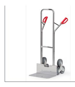
Aluminium tube with aluminium blades, handy welded construction. Safety handles. Aluminum sheet shovel mountable. With 2 three-armed wheel spiders, each equipped with 3 TPE tyres 160 mm Ø. Curved top bar and transversal struts. For safe transport of circular items such as rolls, cans, buckets etc. Flat packed delivery.
