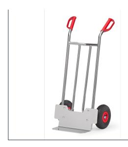
Aluminium trucks made of tubular aluminium with alu blades, very light and handy to use. Aluminum sheet shovel mountable, therefore exchangeable. Pneumatic tyres on synthetic rims, hubs with roller bearings. Flat packed delivery.
