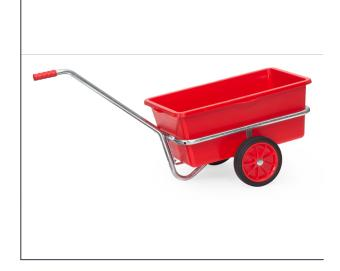
Light hand cart made of tubular steel, welded and galvanised. Suitable for outdoor area. Shaft can be screwed on. With Red plastic tray. Tray 90 liters content, L x W x H =  $715 \times 420 \times 320$  mm. Wheels with solid rubber tyres. Hubs with roller bearings. Flat packed for easy self assembly.
