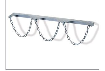
Wall mounting for 3 steel bottles with a diameter of 320 mm. Steel sheet construction, hot-dip galvanised. With security chain and bores for wall mounting.
