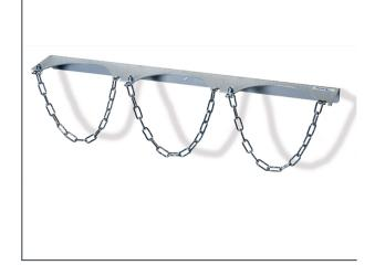
Wall mounting for 3 steel bottles with a diameter of 230 mm. Steel sheet construction, hot-dip galvanised. With security chain and bores for wall mounting.
