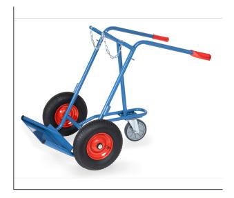
Welded and powder coated blue RAL 5007, tubular steel design. Bottle support with safety chain. Wheels with pneumatic tyres, hubs with roller bearings. For 2 bottles, each 40-50 litres contents,  $\emptyset$  204-229 mm. Receptacle for welding wire. With one additional supporting castor wheel, TPE tyres, 200 x 40 mm.
