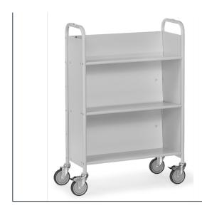
Modular system: Office trolley with shelves inclined to the rear. Back wall in a right angle to the shelf. Inclination approx. 27 mm. Bolted, tubular steel construction, powder coated light grey RAL 7035. Shelves and panels made of derived material timber board, pale grey. 4 swivel castors with TPE tyres, hubs with roller bearings. 2 swivel castors with wheel locks, according to the European Standard EN 1757-3 (safety of platform trolleys). Flat packed for easy self assembly.
