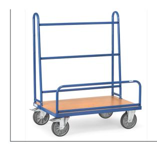
Tubular steel and profile steel welded, powder coated blue RAL 5007. Platform made of derived timber material board, surface beech grain. Bolted tubular steel superstructure. 2 swivel and 2 fixed-wheel castors, TPE tyres, hubs with groove ball bearing. Swivel castors with wheel locks, according to the European Standard EN 1757- 3 (safety of platform trolleys). Effective height: 1050 mm, Height retaining bracket: 300 mm.
