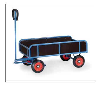
Made of tubular steel, welded and powder coated. Rail 250 mm high, platform, sides and ends made of water-resistant plywood. Bogie steering with shaft and handle. Wheels with solid rubber tyres, hubs with roller bearings. Shaft with safety handle and with an automatic damped retraction in resting position. With automatic braking system effective on the front wheels according to the European Standard EN 1757-3.
