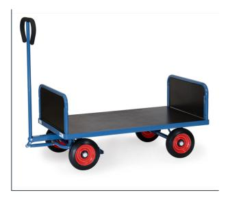
Made of tubular steel, welded and powder coated blue RAL 5007. Platform made of waterresistant plywood. With two ends 300 mm high. Tubular steel frame with waterresistant plywood. Bogie steering with shaft and handle. Wheels with solid rubber tyres, hubs with roller bearings. Shaft with safety handle and with an automatic damped retraction in resting position. With automatic breaking system effective on the front wheels according to the European Standard EN 1757-3.
