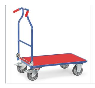
Tubular steel cart, powder coated. Derived timber material boards with coloured plastic surface. Handlebar foldable onto platform. 2 swivel and 2 fixed-wheel castors, TPE tyres, hubs with groove ball bearing. Swivel castors with wheel locks, according to the European Standard EN 1757-3 (safety of platform trolleys).
