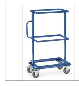
Tubular steel and steel section construction, powder coated. With open frames without board. Capacity upper and middle shelf 50 kg. 2 swivel and 2 fixed-wheel castors, TPE tyres, 125 x 32 mm, hubs with groove ball bearing. Swivel castors with wheel lock, according to European Standard EN1757-3 (safety of platform trolleys).
