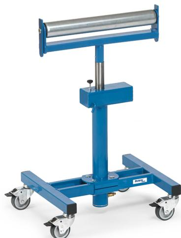
To support long materials on saws, presses, drills etc. Continuously adjustable in height, rotatable and lockable, with pneumatic lowering damping. Mobile. Supporting roller of tubular steel 60 mm Ø, 450 mm wide, ball bearing mounted. Loose gravity-stops on both sides 20 mm above top edge of roller (automatically turn away for wide work pieces). 4 swivel castors, all 4 with wheel locks. Flat packed for easy self assembly.
