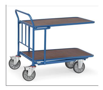
Tubular steel construction, powder coated, platform made of anti-skid waterproof plywood boards. 2 swivel and 2 fixed-wheel castors, TPE tyres. Swivel castors with wheel locks, according to the European Standard EN 1757-3 (safety of platform trolleys).
