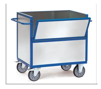
Tubular steel and profile steel welded, powder coated blue RAL 5007. Platforms made of sheet steel, powder coated or galvanized. Sheet steel box cart, angle steel construction, with sides of galvanized steel plates, glued in place. Useful height: 816 mm. 2 swivel and 2 fixed-wheel castors, TPE tyres, hubs with groove ball bearing. Swivel castors with wheel locks, according to the European Standard EN 1757-3 (safety of platform trolleys).
