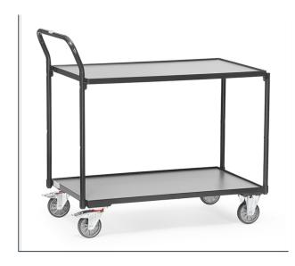
Modular system: Tubular steel welded and powder coated, surface durably protected, resistant to impact and scratches. 2 shelves made of derived timber material boards, in a frame of angle steel, height of rim 12 mm. 2 swivel and 2 fixed-wheel castors, TPE tyres, hubs with groove ball bearing. Swivel castors with wheel locks, according to the European Standard EN 1757-3 (safety of platform trolleys). Capacity upper shelf 80 kg.
