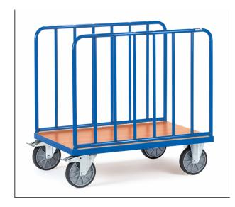
Tubular steel and profile steel welded, powder coated, surface durably protected, resistant to impact and scratches. Platform made of derived timber material boards, surface beech grain. 2 tubular steel side frames with intermediate uprights at intervals of approx. 130 mm. 2 swivel and 2 fixed-wheel castors, TPE tyres, hubs with groove ball bearing. Swivel castors with wheel locks, according to the European Standard EN 1757-3 (safety of platform trolleys).
