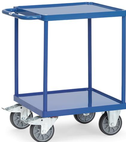
Modular system: Tubular steel and sectional steel, welded and powder coated, surface durably protected, resistant to impact and scratches. 2 square platforms, trays made of steel sheet, with rim 10 mm high, welded oil-tight, powder coated. 2 swivel and 2 fixed-wheel castors, TPE tyres, hubs with groove ball bearing. Swivel castors with wheel locks, according to the European Standard EN 1757-3 (safety of platform trolleys). Capacity upper shelf 200 kg.
