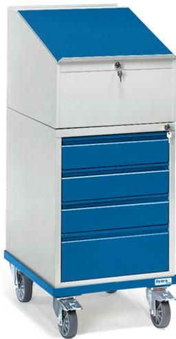
Cupboard of drawers, centrally lockable, 3 drawers 120 mm high and 1 drawer 180 mm high. Ball pull-out and pull-out lock. Fit-on desk-top made of powder-coated steel plate. Desktop foldable. 4 swivel castors with TPE tyres, hubs with groove ball bearing. 2 swivel castors with wheel locks. Powder coated, carcass grey RAL 7035, front blue RAL 5007. Height of surface: 1034/1197 mm, total length: 650 mm, total width: 550 mm. Capacity per drawer 25 kg.
