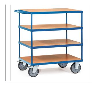
Modular system: Tubular steel and sectional steel, welded and powder coated, surface durably protected, resistant to impact and scratches. 3 shelves made of derived timber material boards, surface beech grain. 2 swivel and 2 fixed-wheel castors, TPE tyres, hubs with groove ball bearing. Swivel castors with wheel locks, according to the European Standard EN 1757-3 (safety of platform trolleys). Capacity upper and middle shelf 200 kg.
