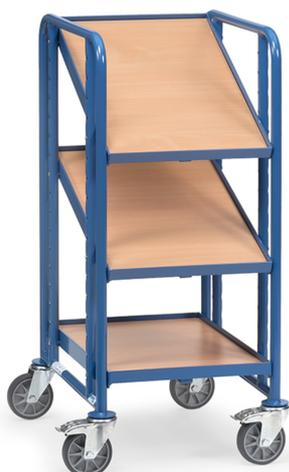
Tubular and sectional steel construction, bolted, powder coated. With 3 platforms with derived timber material boards, rim 10 mm high. Variable use of shelf frames, distance 50 mm, angle when inclined up to 15° and 30°. 4 swivel castors with TPE tyres, hubs with groove ball bearing. 2 Swivel castors with wheel locks, according to European Standard EN1757-3 (safety of platform trolleys). Capacity upper and middle shelves 80 kg.
