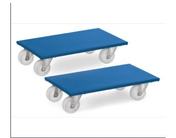
With platform made of beech plywood, with non-slip coating. 4 castors with polyamide wheels 100 x 30 mm. Packing unit = 2 pieces.
