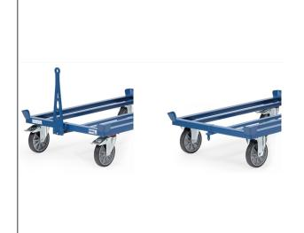
For the transport with towing vehicles up to 6 km/h. Transports up to 5 pallet dollies possible. Maximum train weight 2000 kg. Shaft made of sheet steel. Shaft raises automatically via gas springs into vertical resting position. Robust coupling pin on the fixed-wheel side. Connection via foot operation possible.
