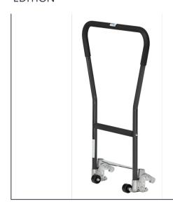
Self-locking push handle for pallet dollies. For comfortable and ergonomic moving of empty and loaded pallet dollies. Sturdy tubular steel construction with strong support claws. Handle and cross tube with softgrip. In unlocked position movable via two auxiliary rollers. Utility patent 20 2014 010 367
