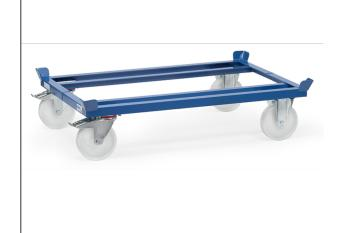
For pallets and boxes. Sturdy sectional steel construction with 4 catch corners for stacking, powder coated. 2 swivel and 2 fixed- wheels 200 x 50 mm. Swivel castors with wheel lock, according to the European Standard EN 1757-3 (safety of platform trolleys). Polyamide wheels, hubs with roller bearings. Low rolling resistance, high chemical resistance, non marking. Road noise. Optional extras are only delivered in a set with pallet dollies because they are welded together.
