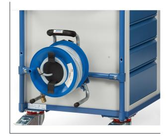
Drum for compressed air hose as a mounting kit for MultiVario table top carts 700 mm wide. Powder-coated blue RAL 5007. Easy assembly to the support tubes of the carts with clamps. 20 m hose, type NW 9. Lockable with padlock (not included in delivery). For models 2402, 2402B, 2402W, 2422, 2442, 2432, 2474, 2475, 2476, 2502, 2502B, 2562, 8102, 8202, 8302, 8242, 8342, 8122, 8222, 8322, 8462
