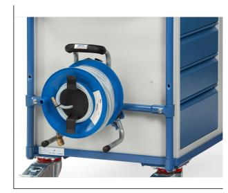
Drum for compressed air hose as a mounting kit for MultiVario table top carts 500 mm wide. Powder-coated blue RAL 5007. Easy assembly to the support tubes of the carts with clamps. 20 m hose, type NW 9. Lockable with padlock (not included in delivery). For models 2400, 2400B, 2400W, 2420, 2500, 2500B, 2560, 8100, 8200, 8240, 8120, 8220
