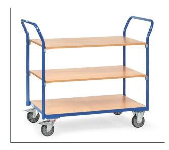
Modular system, platform and pushbar with screw connection, upper shelves can be inserted. Capacity upper and middle shelf 80 kg. Disassembled on delivery. Welded tubular or sectional steel construction, powder coated, blue RAL 5007. Shelves made of derived timber material board, beech decor surface. 2 swivel and 2 fixed-wheel castors, TPE tyres, hubs with groove ball bearing. Swivel castors with wheel locks, according to the European Standard EN 1757-3 (safety of platform trolleys).
