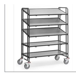
Modular system: Tubular and sectional steel construction, bolted, powder coated anthracite grey RAL 7016. Variable use of shelf frames, distance 100 mm, angle when inclined 15° and 30°. With 5 platforms made of derived timber material boards grey, rim 10 mm high. 4 swivel castors with TPE tyres, hubs with groove ball bearing. 2 Swivel castors with wheel locks, according to European Standard EN1757-3 (safety of platform trolleys). Capacity upper and middle shelves 80 kg.
