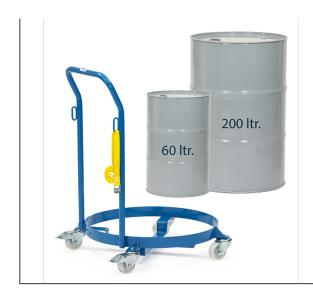
For upright transport of 60 litre or 200 litre steel drums. Welded steel construction, powder coated, blue RAL 5007. Interior-Ø 610 mm. 4 swivel castors, 2 with wheel lock. Wheels made of polyamide. Hubs with glide bearing. Handle screw-on type, with 2 eyelets and 1 clamping band.
