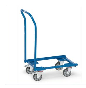
Compatible for Euro boxes 600 x 400 mm, powder-coated blue RAL 5007. Open angle steel construction with tubular push bar. The face end of the frame opposite the push bar is open (without rim), so that boxes can be drawn on or off. 4 swivel castors, TPE tyres. 2 swivel castors with wheel locks, according to the European Standard EN 1757-3 (safety of platform trolleys). Flat packed delivery.
