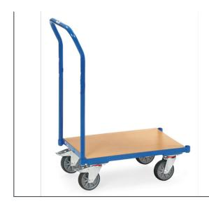
Suitable for Euro boxes,  $600 \times 400$  mm, powder coated, blue RAL 5007. With platform made of derived timber boards, flush with frame. 4 swivel castors, TPE tyres. 2 swivel castors with wheel locks, according to the European Standard EN 1757-3 (safety of platform trolleys).
