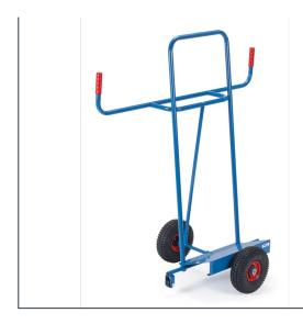
For longitudinal transport of bulky wooden boards and plastic sheets. Tubular steel construction with steel sheet blade, powder coated blue RAL 5007. Wheels with solid rubber tyres. Hubs with roller bearings. 2 support wheels 50 mm Ø. For the longitudinal transport of large-area wooden and plastic panels. Flat packed delivery.
